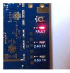
Once 1\_10 illuminates, within 5 seconds remove power from 1\_11. 1\_10 will then extinguish and the flash will be completely erased within 5 seconds. After waiting the full 5 seconds, power cycle the board (it is not sufficient to perform a reset) and the device will be back in a virgin state able to be programmed through the SWD.
