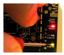
Use a probe with a series resistance to apply power to 1\_11. Then apply power to the board or perform reset. 1\_10 will illuminate indicating beginning of the erase sequence.
